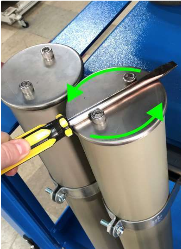
Figure 6.5: Cap removal with Screwdriver
