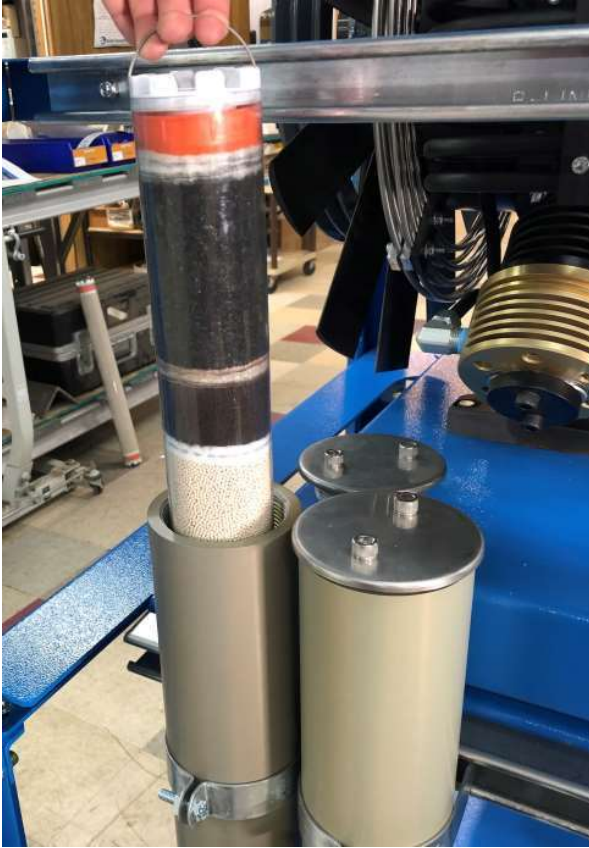
Figure 6.7 Filter cartridge removal.
