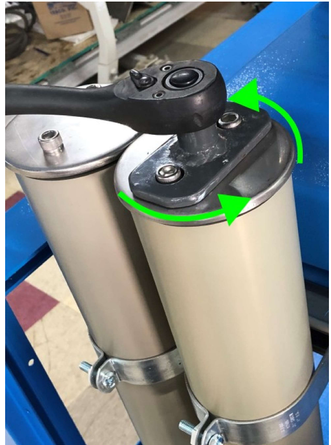
Figure 6.4: Cap Removal with Filter Wrench
