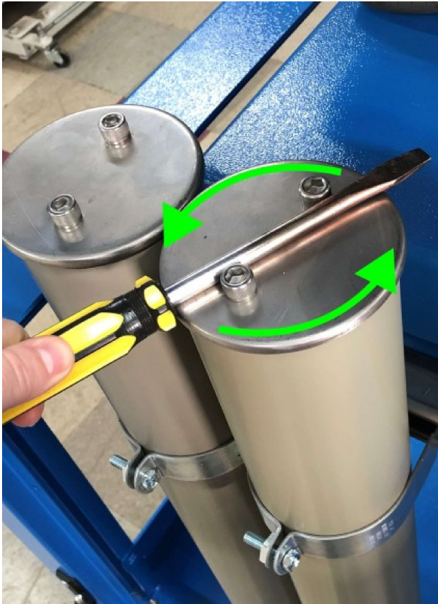
Figure 6.3: Cap removal with Screwdriver
