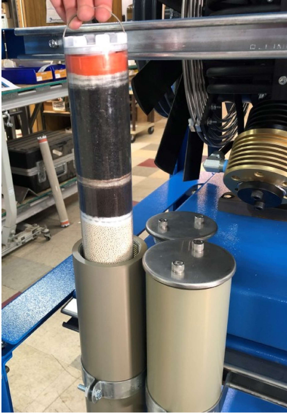
Figure 6.5 Filter cartridge removal.
