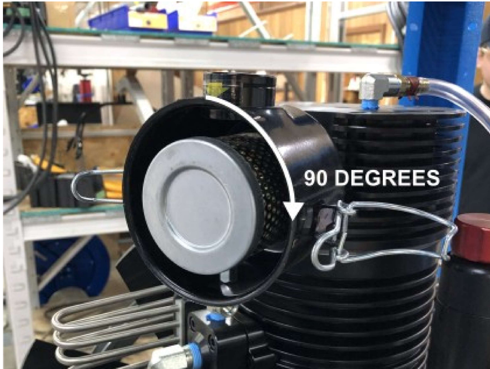
Figure 6.7: Air Intake filter rotation
