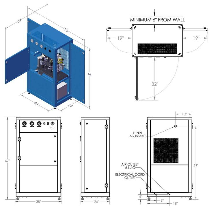
All Arctic Compressors include an 8ft electrical cord and plug. See table for required receptacle size.
