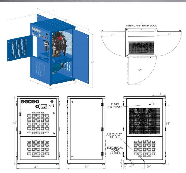
All Arctic Compressors include an 8ft electrical cord and plug. See table for required receptacle size.
